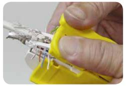
6. Clamp down to close the adapter cap onto the adapter body.
