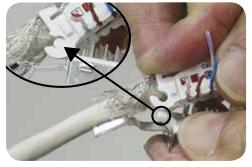
4. Connect the cap hinge to the axis beam of the housing. If correctly connected, the wired cap can rotate back and forth.
