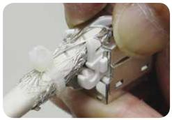
10. Push the shield cover into place, securing the shield cap to the competed assembly.
